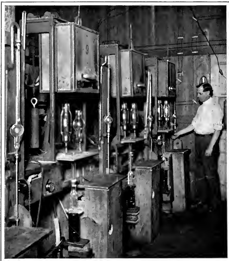
MAKING MODERN VACUUM TUBES
